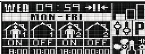
An example of the programmed calendar (working days). The device will be switched on at 8 a.m. and it will be switched off at 10 a.m. It will be switched on again at 6 p.m. and it will be switched off at 12 a.m. The cycle shall be repeated from Monday to Friday.
